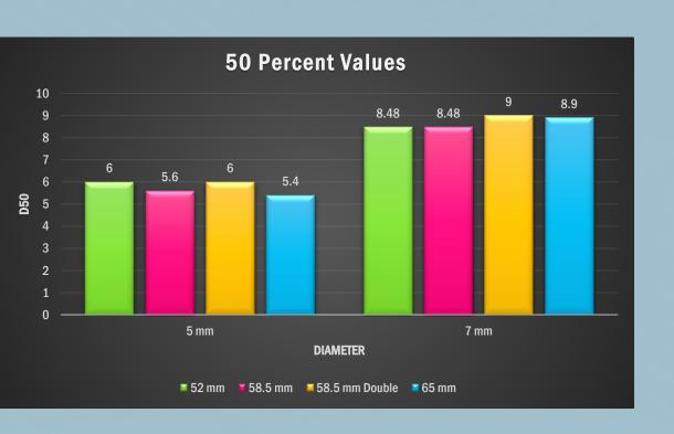
After the extensive testing I have done, I have come to the conclusion the vortex finders with the larger inlet diameter yields better results than the ones with the smaller diameter. The amount of ultrafine particles carried to the underflow stream is far lower when we used the 7mm vortex finder as opposed to the 5mm vortex finder.
