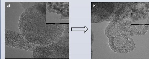
HRTEM images showing a) nascent carbon structure, and b) its change upon partial oxidation. The coarser structure observed along the particle perimeter is “visual” evidence of nanostructure change due to oxidation and corresponding increase in active (edge) sites (as per XPS) as lamellae regress in size.
