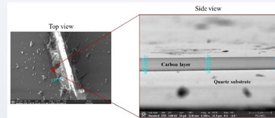
SEM images showing deposited carbon upon quartz substrate; top view (left) and side view (right).
