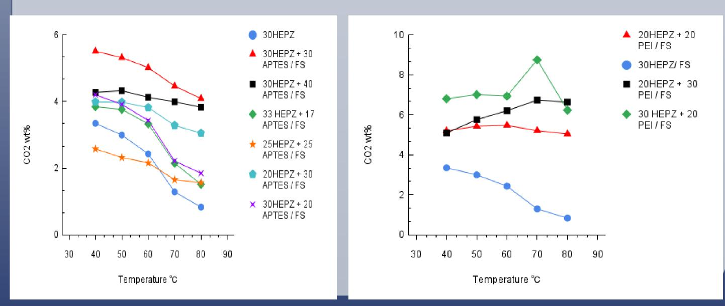
Holding the HEPZ at 30 wt%, we can see that if added in APTES, the more wt% of APTE the higher the material absorb CO2, but slightly decline when APTES is 40 wt%. And for holding the APTES not change, which is the result from 30/30 and 20/30, it still shows that the higher the HEPZ is, the CO2 absorb more. However, we can see the 25/25 lower than everyone, and if we change the HEPZ and APTES in convertibly(one up one down 33/17 and 20/30) the CO2 absorb more.
