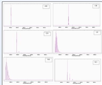
Figure 4. Examples of plasma emission spectra from OH (A-X), CH (A-X), CN (A-X), CF (A-X) and NO (A-X) radicals between 200 – 900 nm.
