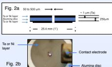
Figure 2. Micro-hollow glow discharge (MHGD) element: (a) schematic (b) photograph of nickel coated alumina disc.
