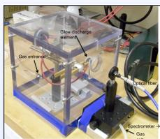
Figure 1. Breadboard test system for micro-hollow cathode in glow discharge mode.
