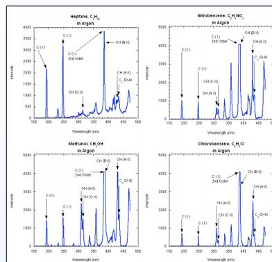
Figure 5. Spectra of model analytes tested in continuous operation
