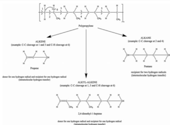
Products of a pyrolysis with Polypropylene (4)
